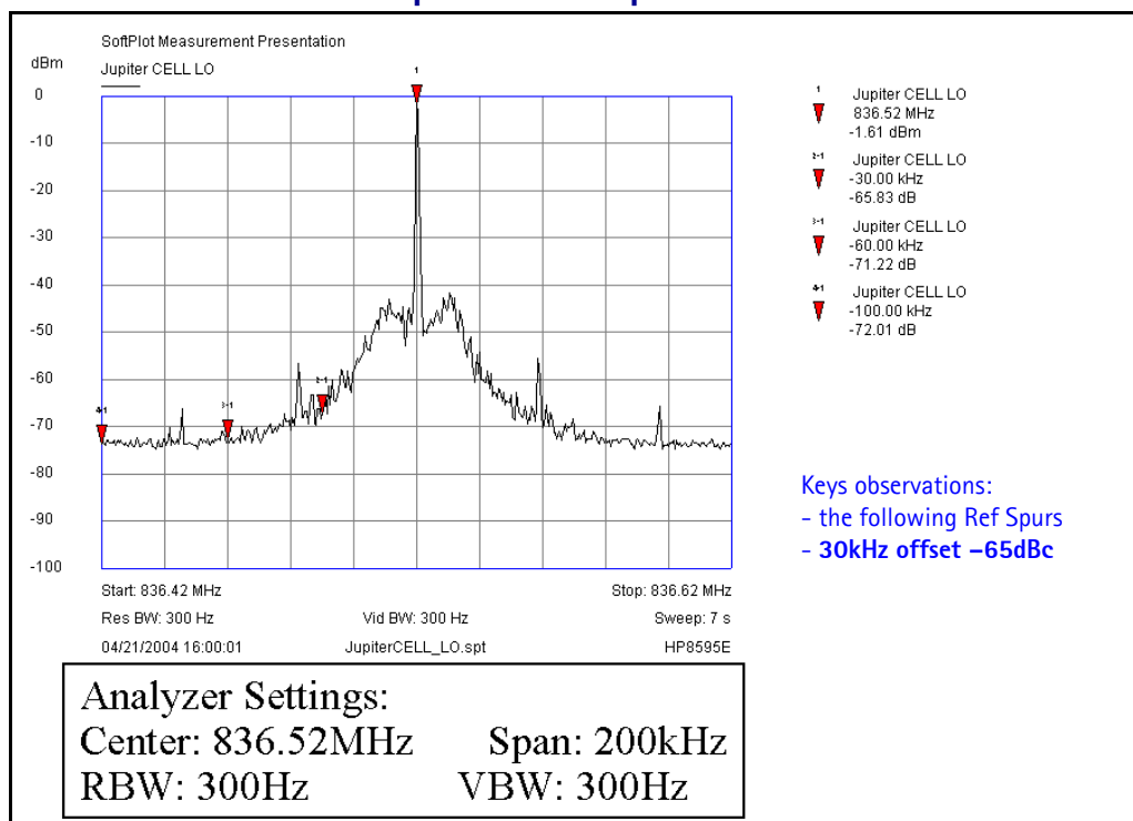
Figure 58: Transmitter UHF LO (3296.16~3395.88)/4 MHz Output for Cell
